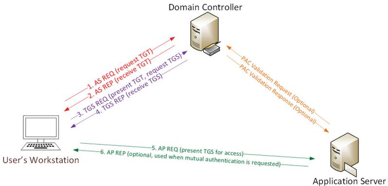
**Figure 7-1:** The KERBEROS authentication process (diagram courtesy of Sean Metcalf and [adsecurity.org](http://adsecurity.org))
