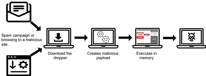
**Figure 3-1:** Fileless attacks often use a dropper to deliver a malicious payload that executes in memory.
